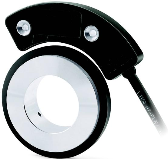
SGSM is a modular and bearingless incremental encoder designed for simple and safe motor speed feedback, angular measurement and motion control in both rotary and linear applications even in demanding and harsh environments. The magnetoresistive sensor and the miniaturized circuitry are fully integrated into a rugged and hermetically encapsulated housing made of Macromelt®. It is also available in redundant SGSD version. SGSM has to be used with MRI/72 magnetic ring.
